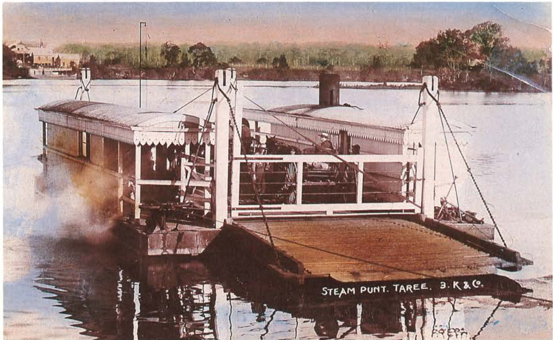
Steam punt across the Manning River at Taree. Travellers on the north coast encountered similar punts at many river crossings along the Pacific Highway. The Manning was not bridged at Taree until 1940. Postcard, c1890.
